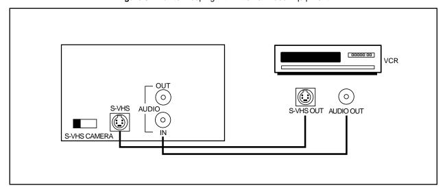
Figure 4. S-VHS Video (Y/C) Input Connections
